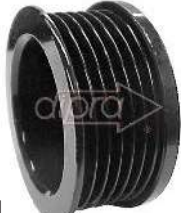
M0104 6 VIAS, MERCEDES BENZ, VW, ETC, .A: 68.0-B: 46- C: 17.0-D: 30.0-E: 62.0
