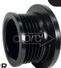
M0132R 5 VIAS -2 Ø exterior, RENAULT CLIO 2, A: 58.5, 76- B: 42.0-C: 17.0-D: 40.0-E: 55.0
